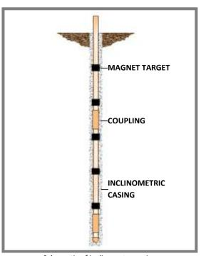
Schematic of inclinometer casing with magnetic targets
